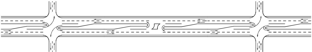
Figure 40. Combination C3—Directional midblock median opening between four-leg intersections with conventional median openings.
