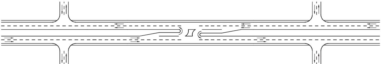
Figure 41. Combination C4—directional midblock median opening between four-leg intersections without median openings.
