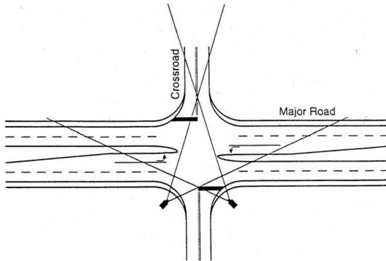
Figure 46. Typical data collection setup using video cameras (8).
