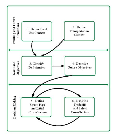
Figure 3.1. The Six-Step process for Applying Charlotte's Urban Street Design Guidelines.
